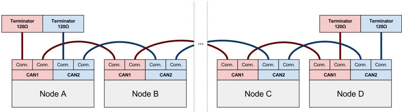
A device that features redundant CAN bus interfaces can be used in a non-redundant CAN bus configuration. In this case, only the first CAN bus interface must be used, and the redundant interfaces should be simply left unconnected, unless the user manual instructs otherwise.
