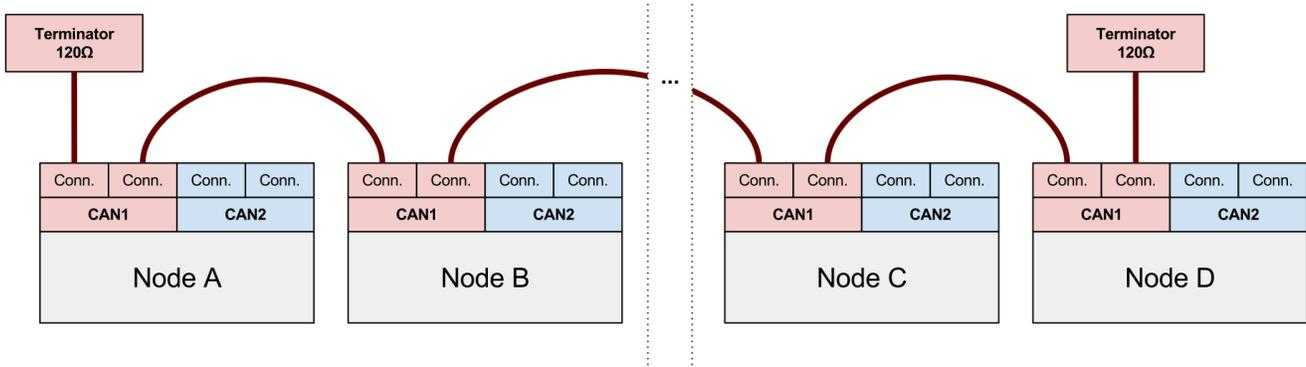
If the device incorporates redundant CAN interfaces, the CAN bus connection circuitry prevents direct current flow between power inputs from different interface connectors, so that if one bus suffers a power failure (e.g., a short circuit), it won't affect the other bus. The power inputs of all available interfaces are always protected by a self-recovering fuse or some other overcurrent protection circuit.
